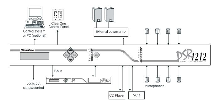
Figure 2.1. PSR1212 installation diagram
